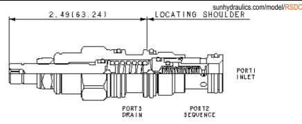
Pilot-operated, balanced piston sequence valves will supply a secondary circuit with flow once the pressure at the inlet (port 1) has exceeded the valve setting. The pressure setting of a sequence valve controls the pressure at port 1 relative to the pressure at the drain (port 3). These valves are insensitive to back pressure at port 2 (sequence), up to the valve setting. They may be used to regulate pressure in place of 2-port relief valves if there is pressure in the return line.
