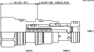
These unbalanced, pilot-to-close logic valves are 2-way switching elements that are spring biased closed. Pressure at either work port 1 or 2 will oppose the spring and tend to open the valve while pressure at port 3 will tend to close it. The force generated at port 3, plus the spring force, must be greater than the sum of the forces acting at port 1 and port 2 for the valve to remain closed. NOTE: The pilot area (port 3) is 1.8 times the area at port 1 and 2.25 times the area at port 2.
