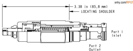
Pilot-operated, anti shock relief cartridges limit maximum system pressure and also limit the rate of pressure rise. The valve opens and then ramps closed at a constant speed, independent of settings and flows. The adjust screw determines the maximum (relief) setting and the minimum (threshold) setting.
