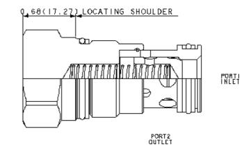
Free-flow, nose-to-side check valves are on/off circuit components that allow free flow from the inlet (port 1) to the outlet (port 2) and block flow in the opposite direction.
