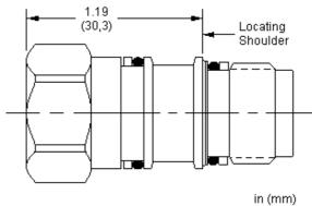
This cavity plug allows ports 1 and 2 to remain open and blocks port 3.
