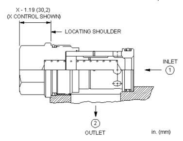
Free-flow, nose-to-side check valves are on/off circuit components that allow free flow from the inlet (port 1) to the outlet (port 2) and block flow in the opposite direction.
