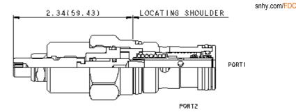
Fully adjustable, pressure-compensated flow controls with reverse-flow check provide precise flow regulation for meter-in or meter-out applications where there may be wide pressure fluctuations. They are infinitely adjustable from nearly closed up to the maximum flow. An integral high-capacity check valve provides unrestricted flow from port 2 to port 1.
