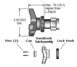
Sun now offers its latest in hand knob control. This ergonomically designed, tri-grip handknob incorporates dual functionality in one package. It can be used to achieve full range control (five turns) or can be used to limit the maximum allowable setting.
