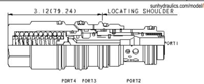
Vented, balanced load control valves combine a balanced modulating element with a reverse flow check. The check valve allows free flow from the directional valve (port 2) to the load (port 1) while the pilot to open modulating element controls flow from port 1 to port 2. Pilot pressure at port 3 determines the flow setting. Backpressure at port 2 does not affect the flow setting because the spring chamber references the vent (port 4).
