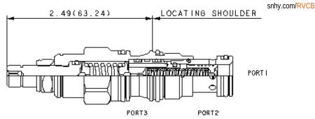
Three-port normally closed modulating elements with relief provide two functions when combined with an external orifice. The mainstage is a bypass compensator that controls a priority flow into the circuit, determined by the external orifice. Input flow in excess of the priority flow is bypassed to tank (port 2). If the inlet (port 1) pressure rises to the valve setting, the valve operates as a normal relief valve.
