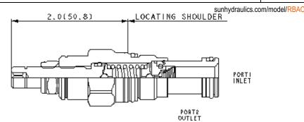
Direct-acting, pilot relief cartridges are used to remotely control the pressure setting of other pilot-operated valves. Because capacity is limited to pilot flow, these valves should be used with other higher flow valves.
