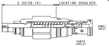
Direct-acting relief cartridges are normally closed, pressure-limiting valves used to protect hydraulic components from pressure transients. When the pressure at the inlet (port 1) reaches the valve setting, the valve starts to open to tank (port 2), throttling flow to limit the pressure rise. These valves are smooth and quiet, essentially zero leak, dirt tolerant, immune to silting and are very fast.
