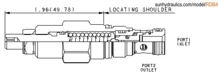
Direct-acting relief cartridges are normally closed, pressure-limiting valves used to protect hydraulic components from pressure transients. When the pressure at the inlet (port 1) reaches the valve setting, the valve starts to open to tank (port 2), throttling flow to limit the pressure rise. These valves are smooth and quiet, essentially zero leak, dirt tolerant, immune to silting and are very fast.
