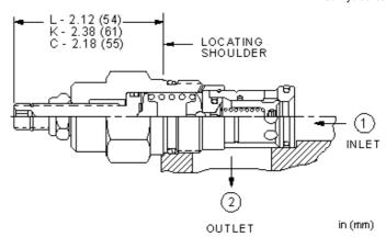
Pilot-operated, balanced-poppet relief cartridges are normally closed pressure regulating valves. When the pressure at the inlet (port 1) reaches the valve setting, the valve starts to open to tank (port 2), throttling flow to regulate the pressure. These valves are accurate, smooth, quiet, fast, and have low pressure rise vs. flow.
