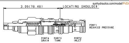
Externally drained, pilot-operated pressure reducing/relieving valves reduce a high primary pressure at the inlet (port 2) to a constant reduced pressure at port 1, with a full-flow relief function from port 1 to tank (port 3). Draining the pilot section at port 4 makes these valves insensitive to pressure at tank (port 3) and provides a means for remote control by pilot or 2-way valves.
