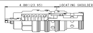
This valve is a 2-way, 2-position proportional throttle. Ports 2 and 3 are normally closed. Pilot pressure at port 1 creates a metering orifice between port 2 and 3 that is proportional to the pressure at 1. The force balance of the flow forces, spring and pilot pressure results in a degree of partial self-compensation as the load pressure changes.
