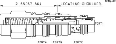
Vented, balanced load control valves combine a balanced modulating element with a reverse flow check. The check valve allows free flow from the directional valve (port 2) to the load (port 1) while the pilot to open modulating element controls flow from port 1 to port 2. Pilot pressure at port 3 determines the flow setting. Backpressure at port 2 does not affect the flow setting because the spring chamber references the vent (port 4).
