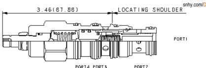
Normally open, pilot-operated, 2-way directional cartridges are switching devices typically used in moderate flow circuits. They can be used by themselves or to actuate larger pilot-operated directional cartridges or logic cartridges. The valve shifts when the pressure differential between port 1 and port 4 exceeds the setting.
