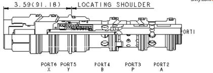
Two-position, 4-way directional cartridges are spring-offset, 6-port directional valves that can be configured from a choice of 9 different spool options. The supply port is port 3 and all ports will accept 5000 psi (350 bar). Capacity for these pilot-to-shift valves is dependent on the spool type specified.
