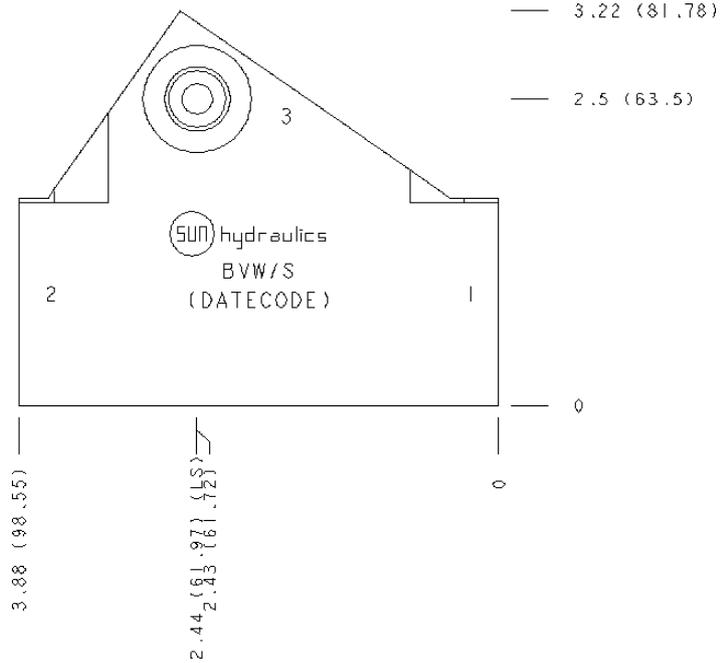
Pilot-operated, balanced-piston relief cartridges are normally closed pressure regulating valves. When the pressure at the inlet (port 1) reaches the valve setting, the valve starts to open to tank (port 2), throttling flow to regulate the pressure. These valves are accurate, have low pressure rise vs. flow, they are smooth and quiet, and are moderately fast.
