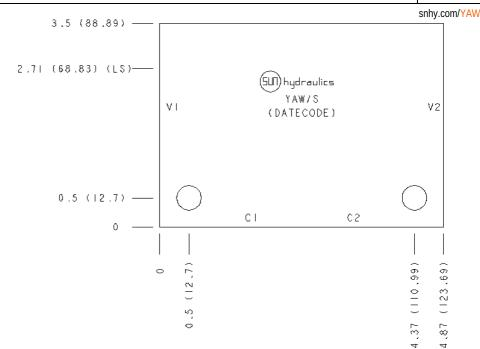
Pilot-operated, balanced-piston relief cartridges are normally closed pressure regulating valves. When the pressure at the inlet (port 1) reaches the valve setting, the valve starts to open to tank (port 2), throttling flow to regulate the pressure. These valves are accurate, have low pressure rise vs. flow, they are smooth and quiet, and are moderately fast.
