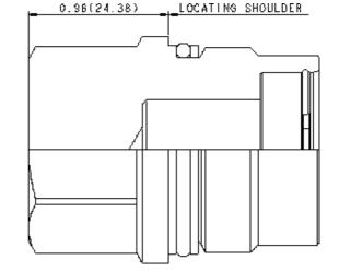
These cavity plugs can be used for both two-port and four-port cavities and allow all ports to remain connected.
