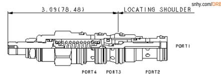
Direct-acting, 3-way directional cartridges (3 to 4 open, 2 blocked) are switching devices typically used in moderate flow circuits. They can be used by themselves or to actuate larger pilot operated directional cartridges or logic cartridges. The valve shifts when the pressure differential between port 1 and port 4 exceeds the setting.
