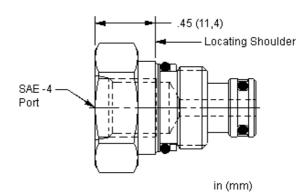
This cavity plug includes an external port open to port 1 and blocks port 2.
