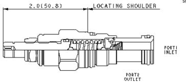
Direct-acting, pilot relief cartridges are used to remotely control the pressure setting of other pilot-operated valves. Because capacity is limited to pilot flow, these valves should be used with other higher flow valves.
