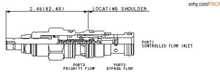
Bypass/restrictive, fixed-orifice, priority flow controls take an input flow at port 1 and use it to satisfy the priority flow at port 3. If the input flow exceeds the priority flow requirement, the excess is bypassed out port 2. The bypass flow may be used in a secondary circuit.
