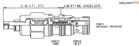
Pilot-operated, pressure reducing/relieving valves reduce a high primary pressure at the inlet (port 2) to a constant reduced pressure at port 1, with a full-flow relief function from port 1 to tank (port 3).
