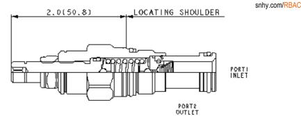
Direct-acting, pilot relief cartridges are used to remotely control the pressure setting of other pilot-operated valves. Because capacity is limited to pilot flow, these valves should be used with other higher flow valves.
