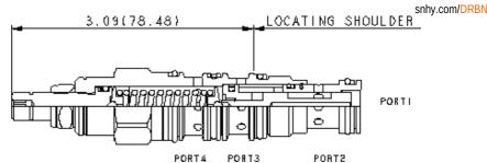
Normally closed, direct-acting, 3-way directional cartridges are switching devices typically used in moderate flow circuits. They can be used by themselves or to actuate larger pilot-operated directional cartridges or logic cartridges. The valve shifts when the pressure differential between port 1 and port 4 exceeds the setting.
