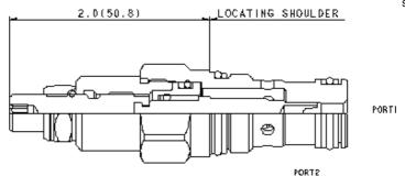
Needle valves are fully adjustable orifices used to regulate flow. They are infinitely adjustable from fully closed up to the maximum orifice diameter. They are not pressure compensated and may be used as flow controls or as shutoff valves.
