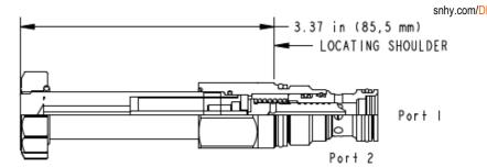
This solenoid-operated 2-way, 2-position cartridge is a direct-acting, balanced spool directional valve. The valve is available in either a normally open or normally closed configuration and is designed to be used with FLeX Series coils.
