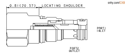
Free-flow, nose-to-side check valves are on/off circuit components that allow free flow from the inlet (port 1) to the outlet (port 2) and block flow in the opposite direction.
