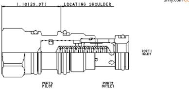
This valve is a spring biased closed, pilot-to-close check cartridge that has a 1.8:1 pilot ratio. The valve allows flow from port 1 to port 2 and blocks reverse flow. Pressure at the pilot port opposes pressure at port 1 at a ratio of 1.8:1. This valve is most often used in regeneration circuits.
