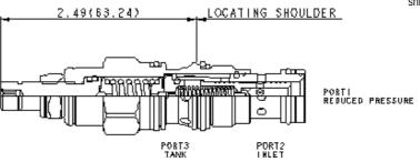
Pilot-operated, pressure reducing/relieving valves reduce a high primary pressure at the inlet (port 2) to a constant reduced pressure at port 1, with a full-flow relief function from port 1 to tank (port 3).
