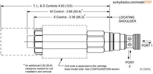
This solenoid-operated 2-way, 2-position cartridge is a direct-acting, poppet-style directional valve. The valve is available in either a normally open or normally closed configuration and is designed to be used with 740 and 747 Series coils.
