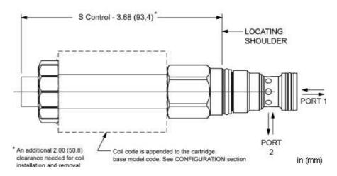
This solenoid-operated 2-way, 2-position cartridge is a direct-acting, balanced spool valve with a soft shift feature. The soft shift feature reduces system shock due to valve actuation. The valve is available in either a normally open or normally closed configuration.
