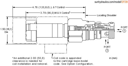
This solenoid controlled, 2-way, 2-position cartridge is a pilot-operated, poppet style directional valve with reverse free flow check. It is available in either a normally open or normally closed configuration. Due to its poppet style construction, it has extremely low leakage.
