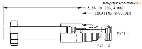
This solenoid-operated 2-way, 2-position cartridge is a direct-acting, balanced spool valve with a soft shift feature. The soft shift feature reduces system shock due to valve actuation. The valve is available in either a normally open or normally closed configuration.
