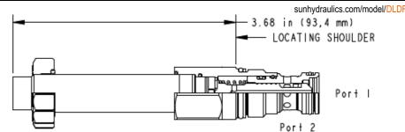
This solenoid-operated 2-way, 2-position cartridge is a direct-acting, balanced spool valve with a soft shift feature. The soft shift feature reduces system shock due to valve actuation. The valve is available in either a normally open or normally closed configuration.
