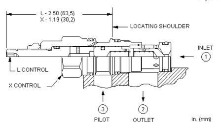
This valve is a spring biased closed, pilot-to-close check cartridge that has a 20:1 pilot ratio. The valve allows flow from port 1 to port 2 and blocks reverse flow. Pressure at the pilot (port 3) opposes pressure at port 1 at a ratio of 20:1.
