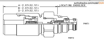
These pilot-stage, directional, 2-position, 2-way valves are hydraulically operated, spring-return cartridges and are available in either a normally open or normally closed configuration. These cartridges are designed for pilot flow applications and utilize Sun's T-8A cavity so they can be used in conjunction with Sun's pilot-operated, main-stage valves.
