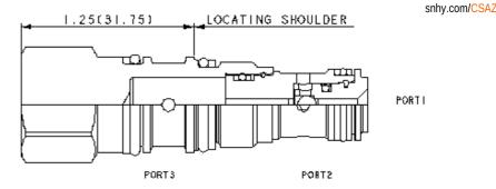
The single ball shuttle connects the higher of two work ports to the signal or common port. The signal is sensed at port 2.
