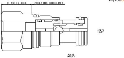
The single ball shuttle connects the higher of two work ports to the signal or common port. It features an external load port located in the hex-end of the cartridge and the signal is sensed at port 2.
