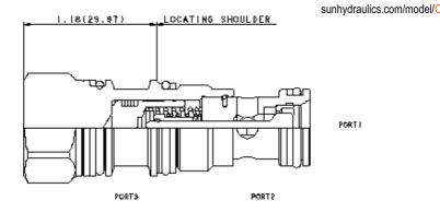
This valve is a pilot to open check valve. It has a non-sealed pilot, a Delrin seat, and is non-vented. It allows free flow from the valve (port 2) to the load (port 1) and blocks flow in the opposite direction. Pressure at the pilot (port 3) will open the valve, allowing flow from port 1 to port 2. Pilot pressure needed at port 3 to open the valve is directly proportional to the load pressure at port 1. Pressure at port 2 directly opposes pilot pressure.
