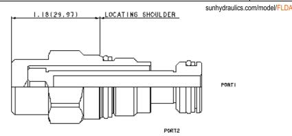
Sun filter elements are available as Surface Type (Last Chance) and Depth Style elements. The flow path is Port 2 to Port 1 and should not be used in reverse, even with a reverse free flow check valve installed. The elements have a high collapse pressure and are intended to be used in line with the system. Filter life will depend on initial system cleanliness and the amount of dirt ingression to the system when operating.
