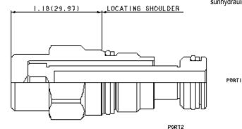
Sun filter elements are available as Surface Type (Last Chance) and Depth Style elements. The flow path is Port 2 to Port 1 and should not be used in reverse, even with a reverse free flow check valve installed. The elements have a high collapse pressure and are intended to be used in line with the system. Filter life will depend on initial system cleanliness and the amount of dirt ingression to the system when operating.
