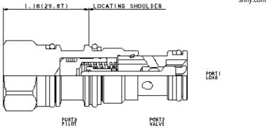
This valve is a pilot to open check valve. It has a non-sealed pilot, a steel seat, and is non-vented. It allows free flow from the valve (port 2) to the load (port 1) and blocks flow in the opposite direction. Pressure at the pilot (port 3) will open the valve from port 1 to port 2. Pilot pressure needed at port 3 to open the valve is directly proportional to the load pressure at port 1. Pressure at port 2 directly opposes pilot pressure.
