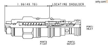
Counterbalance valves with pilot assist are meant to control an overrunning load. The check valve allows free flow from the directional valve (port 2) to the load (port 1) while a direct-acting, pilot-assisted relief valve controls flow from port 1 to port 2. Pilot assist at port 3 lowers the effective setting of the relief valve at a rate determined by the pilot ratio.
