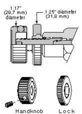
Sun offers a general purpose handknob with lock knob control for use in systems where frequent adjustments are necessary. The handknob components are added to the basic L control. Cartridges may be ordered in this configuration from Sun by specifying a K control in the model number. Sun kits for field conversion are also available.
