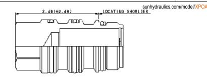
These cavity plugs can be used for both four-port and six-port cavities. When used in four-port cavities (T-21A, T-22A, T-23A and T-24A), ports 1 and 2 remain connected and ports 3 and 4 are blocked. When used in six-port cavities (T-61A, T-62A, T-63A and T-64A), ports 1, 2, 3 and 4 remain connected and ports 5 and 6 are blocked.
